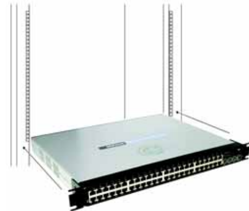
Figure 3-3: Mount the Switch in the Rack
