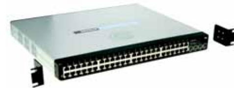
Figure 3-2: Attach the Brackets to the Switch
